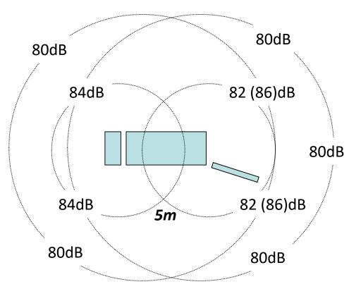
Note – Readings are for guidance only and may vary depending on chassis type and full equipment specifications
